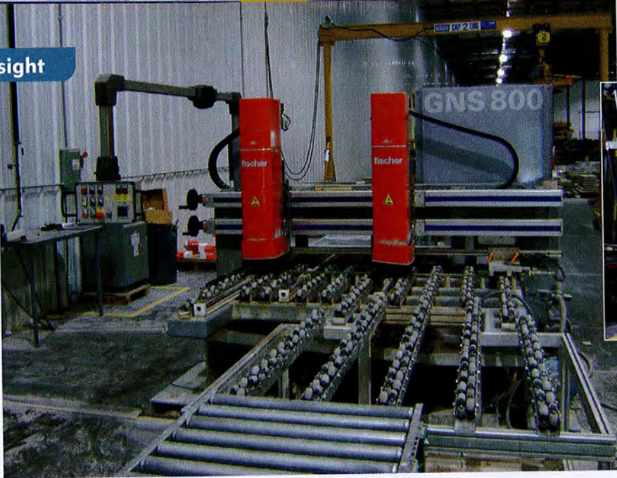
(Left) To set the anchors in the back of the stone panels, ASI installed a Fischer drilling machine and trained employees to use it. (Above) Once the panels were completed, they were shipped by truck to Chicago. (Photos courtesy ASI Limited)
